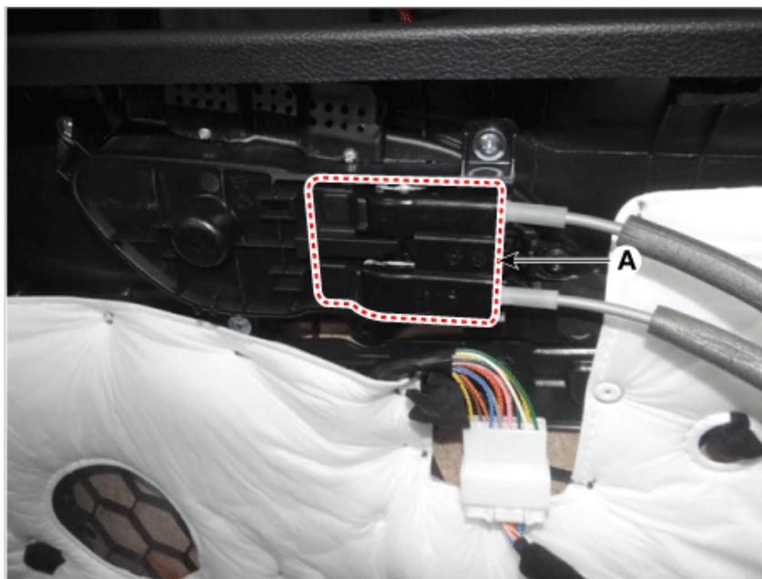
5. Disconnect the power window switch connector (A) and rear door tweeter speaker (B).
