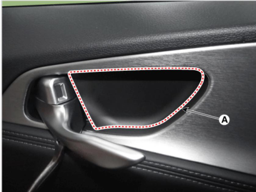
2. Remove the rear door pull handle cap (A) by using a remover.
