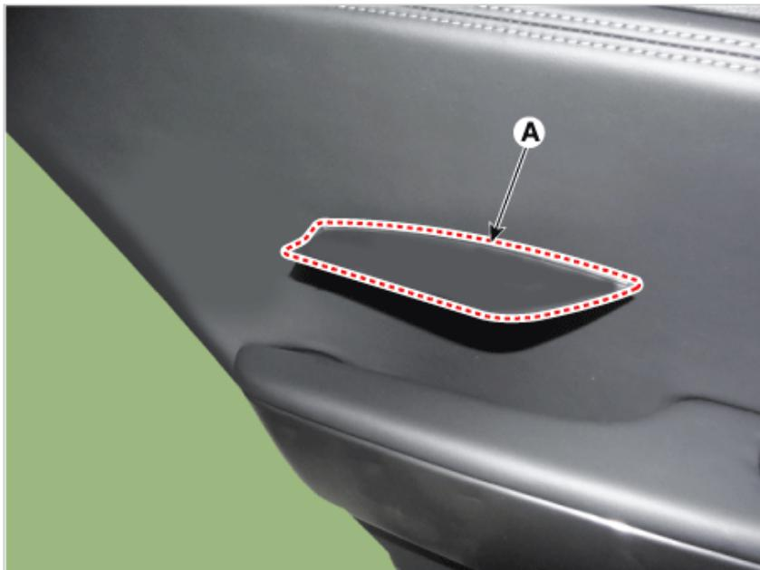
3. Remove the rear door trim (A) after loosening the mounting screw.
